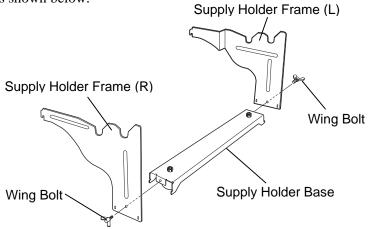
**2.** Attach the assembled Supply Holder Frame to the rear of the B-852 printer by inserting the hooks of the Frame into the two slots in the rear of the printer as shown in the figure below.
